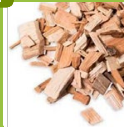
Picture 3. Wood chips as fuel in boilers →
