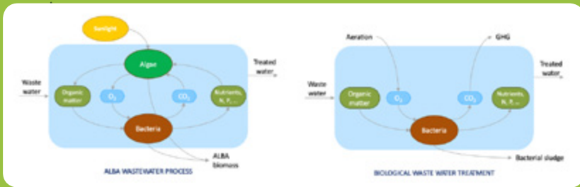
Figure 1. Wastewater treatment with (left) and without algae (right). Source: AlgEn, algal technology center, llc. ↵
